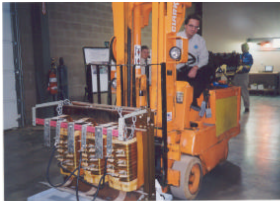
EPRI's fork lift truck, powered by supercapacitors!
