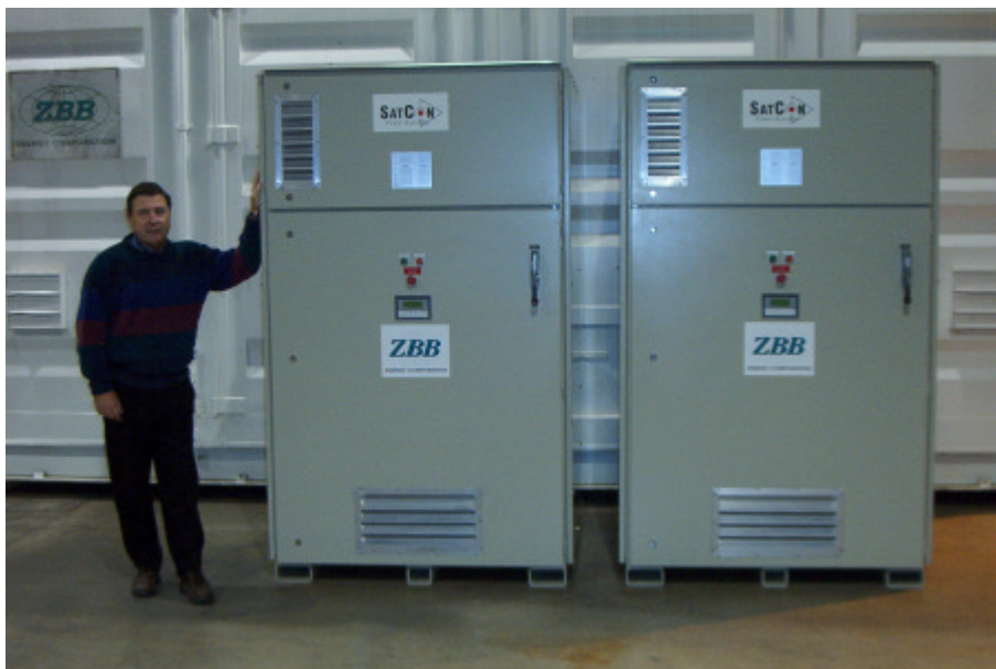
A view inside ZBB's manufacturing plant: two, stand-alone 50 kWh modules with the power electronics built into the upper portion of the cabinet with the zinc bromine battery underneath.
